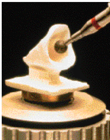
Figure 14-18G: As the pattern is being traced on the left side, the coping is being milled on the right side of the machine. Several new tools, specially designed for crowns and bridges, are used to obtain a precise reproduction of the pattern.
