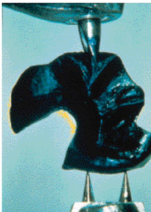
Figure 14–18B: The hardened wax pattern is placed in the scanning, or left side, of the Celay machine. Several different pin configurations are available to hold the different sizes and shapes of patterns.
