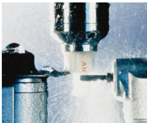
Figure 14-17G: A block of porcelain has been placed into the machine and is now being milled.
