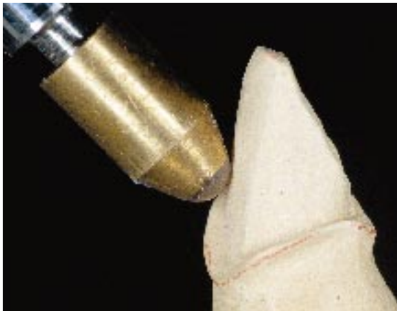
Figure 15–15I: The scanning probe reads every part of the tooth surface and inputs the measurements into the computer. Next the finish line and thickness of ceramic coping is established.
